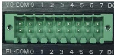
9\*2 PIN, 2.54mm (DI: 8bit, DO: 8bit, DI COM, VCC and GND pins).
