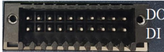
2.54mm 2x10 Terminal Block Including (DI: 8bit, DO: 8bit, DI COM, VCC and GND pins).
